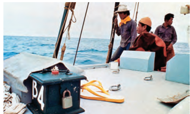
Figure 5. Percy’s patented box is used to store recovered natural pearls on the deck of this pearling lugger. Note the red cap over the opening and the padlock on the door at the front of the box. Photo courtesy of Pas-paley Pearling Co.
