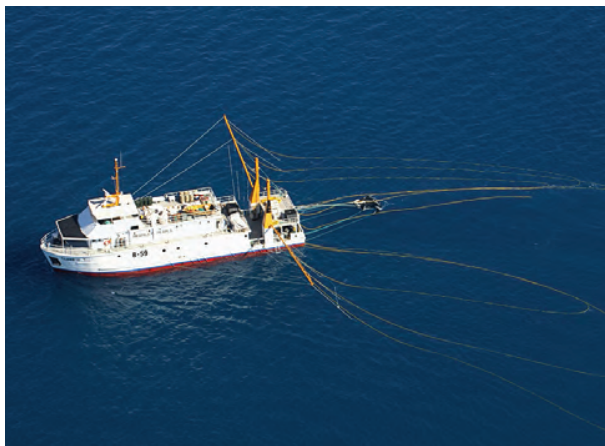
Figure 22. A Paspaley diving vessel operates off Eighty Mile Beach. The lines running from the stern of the vessel are the divers’ air hoses and safety lines. Photo by K. Scarratt.
